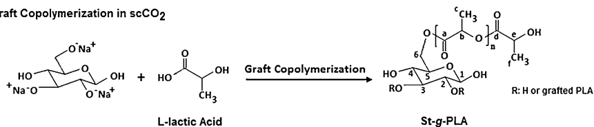
Fig. 1. The synthetic pathway of the St-g-PLA copolymer.
